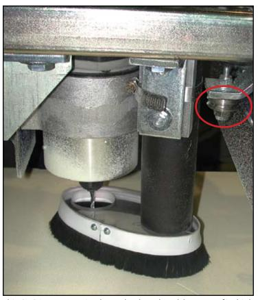
This CNC Router uses DualVee wheels and track because of its high speed capability, accuracy and self-cleaning action.
