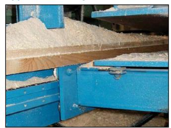
This multi-axis guidance system automatically mills notches in heavy logs used in prefabricated log homes. DualVee components installed in early 2003 are still operating without apparent wear, and without any lubrication on the tracks.
