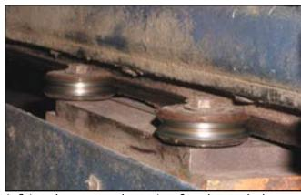
A flying shear exposed to gritty, fine dust and glue uses DualVee, because it forces the debris off the ends of the track like a squeegee. "Five to six million cycles later, it remains a really reliable, simple-to-use system," according to the unit manager responsible for the redesign.
