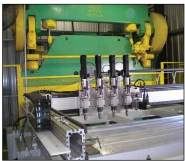
An automated multi-head drilling machine drills successive rows of 112 holes in large sheets. HepcoMotion® HDS Heavy Duty Slide system was selected because it provided the rigidity needed for accuracy.
