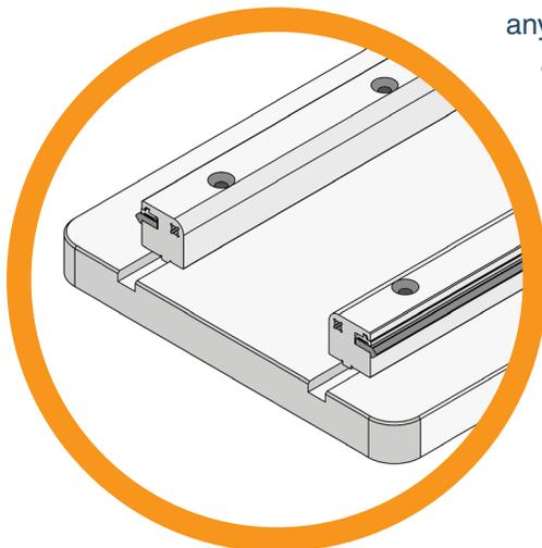
Figure 5. Machined channels
