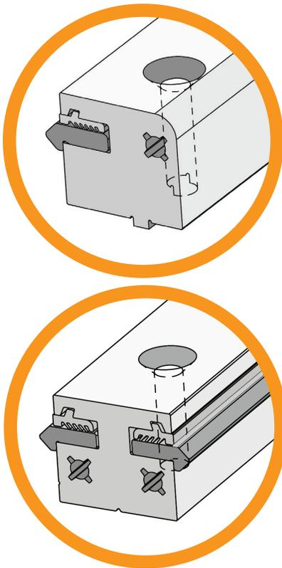
Figure 4. Single-edge and double-edge track
