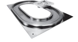
For larger gears, MOD2 teeth up to 8mm, MOD3 teeth up to 12mm, MOD5 teeth up to 20mm, MOD8 teeth up to 33mm, and MOD10 teeth up to 40mm wide are recommended.
