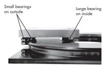
A further useful version of **PRT2 1-Trak** is shown below. In this design, the carriage fits inside a channel-section track which has inward-facing vees that engage the bearings. The advantage of this configuration is that the contact points between bearings and slide vees are spaced very far apart, giving higher moment load capacity and stiffness.
