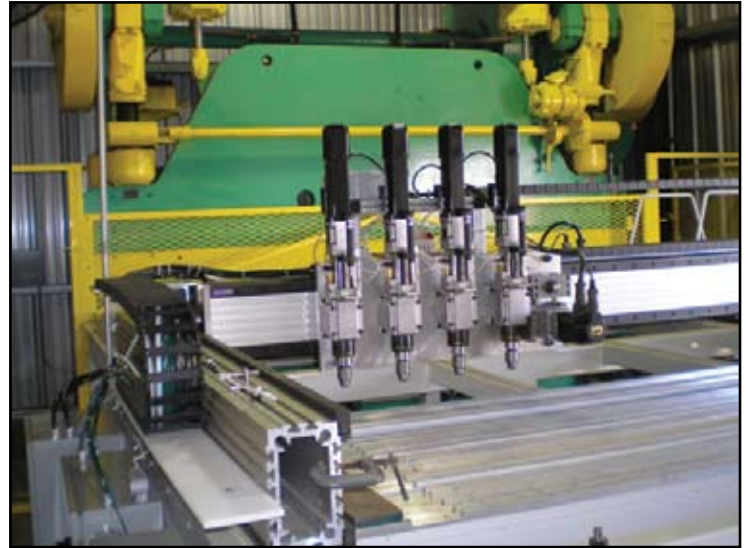
An automated multi-head drilling machine drills successive rows of 112 holes in large sheets. HepcoMotion® HDS Heavy Duty Slide system was selected because it provided the rigidity needed for accuracy.
