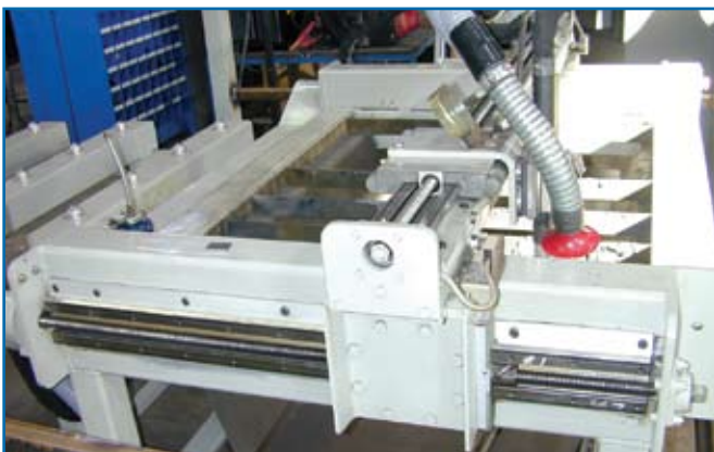
Three ball screw driven LoPro systems are used on this plasma cutter, which operates in a very harsh environment consisting of smoke, abrasive dust, weld spatter, hot sparks, and elevated temperatures.
