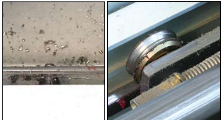
With metal shavings flying, intensified by cutting fluids that help the shavings stick to all surfaces, this CNC turning center uses DualVee wheels and track to move its heavy doors as well as the bar feeder. DualVee stands up to the rigors of constant opening and closing in a high debris environment.
