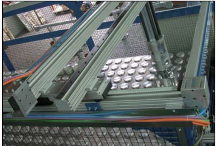
A high duty, high speed pick and place application uses HepcoMotion DLS4 belt driven actuators for the X and Y axes, and HDCB Heavy Duty Compact Beam for the Z axis.
