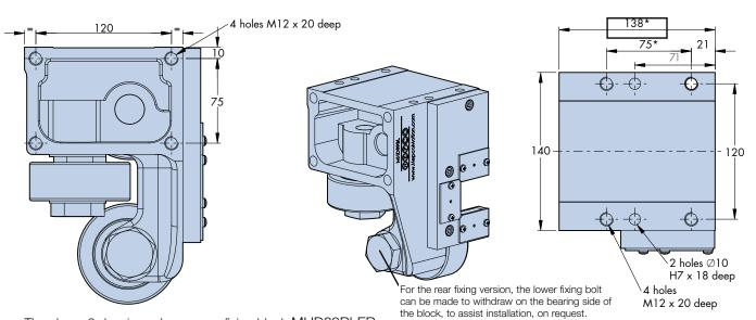
The above 3 drawings show a rear fixing block MHD89BLER
